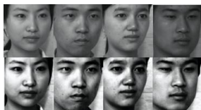
Fig. 1. Result of eliminate the effect of un-even illumination
