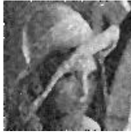
Fig. 8. Result of filtering by medium filter, the size of filter is 3 \times 3
