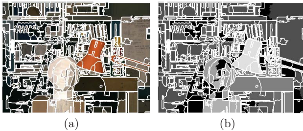
Fig. 1. (a) the segmentation result by the mean shift with embedded edge confidence algorithm. (b) the “uncertain” regions in disparity map after first cooperation.
